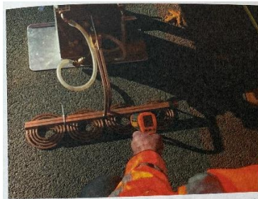
Figure: Self-healing asphalt pavement in the Netherlands is being checked up for the service conditions in five years after it was constructed.
